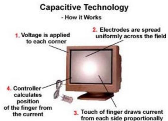
Capacitive type touch screens are very durable, and have a high clarity. They are used in a wide range of applications, from restaurant and POS use to industrial controls and information KIOSKS.
